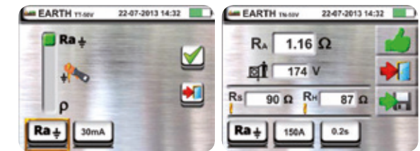
Earth resistance measurement by Volt-ampere method
