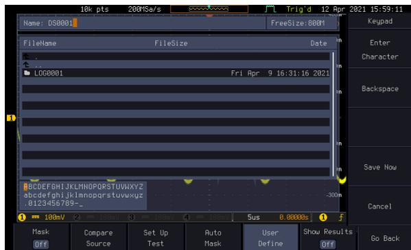
15. Use the *VARIABLE* knob and the select key to change the name of the file if needed and press the *Save Now* button from the side menu to save the user-defined mask.
