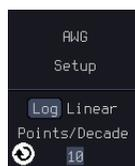
**Example** For the 100-1000Hz decade and 15 points per decade, the frequency sweep step is given by  $(1000-100)/15 = 60\text{Hz}$ , i.e. measurements will be taken at 100Hz, 160Hz, 220Hz, 280Hz, ..., 940Hz.
