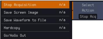
6. Press *Action on Failure On/Off*. The above setting will be executed only when Failure On or Off occurs.
