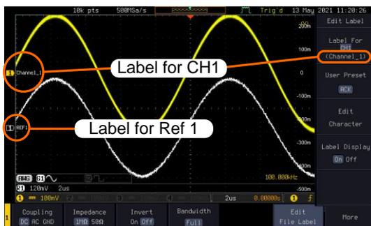
In the example above, the file label for channel 1 is displayed next to the channel indicator and is also displayed in the *Edit Label* menu. The Ref\_1 file label is shown next to the reference indicator.
