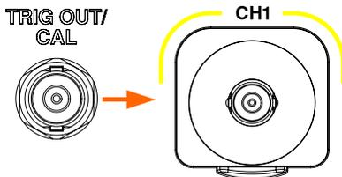
8. Press *Vertical* again after connecting CAL to the channel 1 input.
