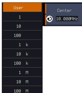
the *VARIABLE* knob can be used to select one. Press again on the *Center* button; the *VARIABLE* knob can now be used to set the frequency in increments of the chosen step resolution.
