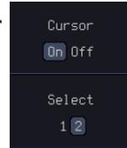
Move the active cursor along the active trace using the *VARIABLE* knob. The corresponding frequency value in Hz (X-axis), gain value in dB (left Y-axis) and phase value in degree (right Y-axis) messages are shown below.
