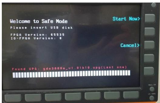
3. When the firmware file of USB flash disk has been recognized by oscilloscope, a message of “Found UPG: xxx.upg” will appear on the lower corner.
