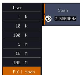
The *VARIABLE* knob can be used to select one. Press again on the *Span* button; the *VARIABLE* knob can now be used to set the frequency in increments of the chosen step resolution.
