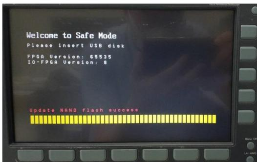
6. Restart the oscilloscope manually. Check the firmware version by pressing the "Utility" → "System" → "System Info". The system information screen that it is being updated.
