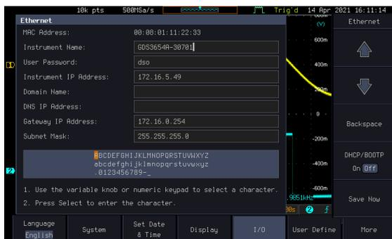
7. Use the Up and Down arrows on the side menu or use the numerical keypad on front panel to navigate to each Ethernet configuration item.
