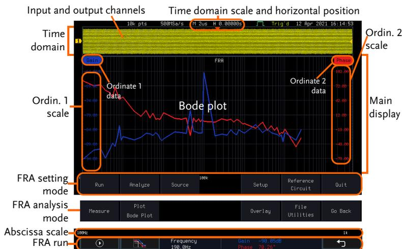
**Introduction**      The FRA application is divided into two main operation modes: Setting and Analysis mode.
