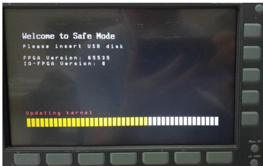
5. When the status indicator shows the complete status (status indicator in yellow completely) and a message of "Update NAND flash success" will appear on the top of status indicator. The firmware upgrading procedure is completed.
