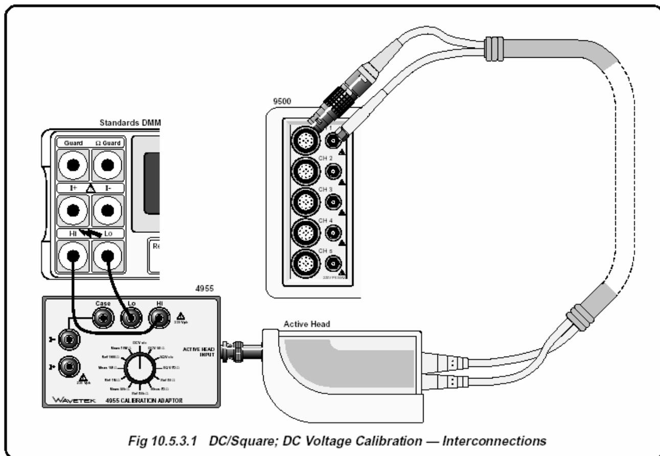
Fig 10.5.3.1 DC/Square; DC Voltage Calibration — Interconnections
