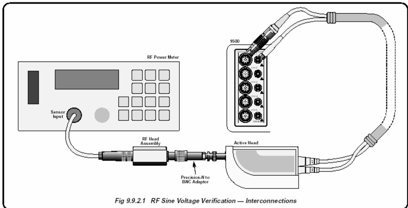
Fig 9.9.2.1 RF Sine Voltage Verification — Interconnections
