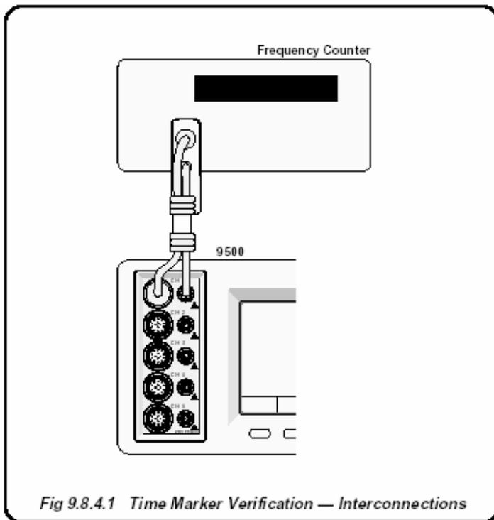
Fig 9.8.4.1 Time Marker Verification — Interconnections
