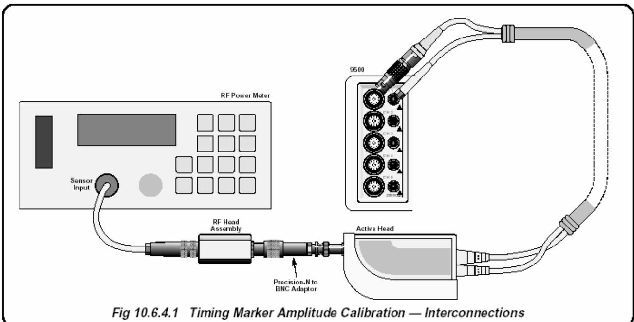
**Fig 10.6.4.1 Timing Marker Amplitude Calibration — Interconnections**
