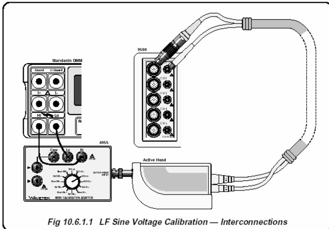
Fig 10.6.1.1 LF Sine Voltage Calibration — Interconnections
