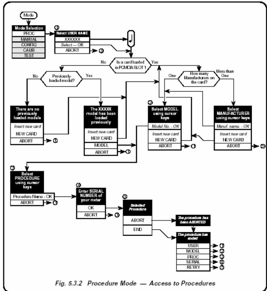
Fig. 5.3.2 Procedure Mode — Access to Procedures
