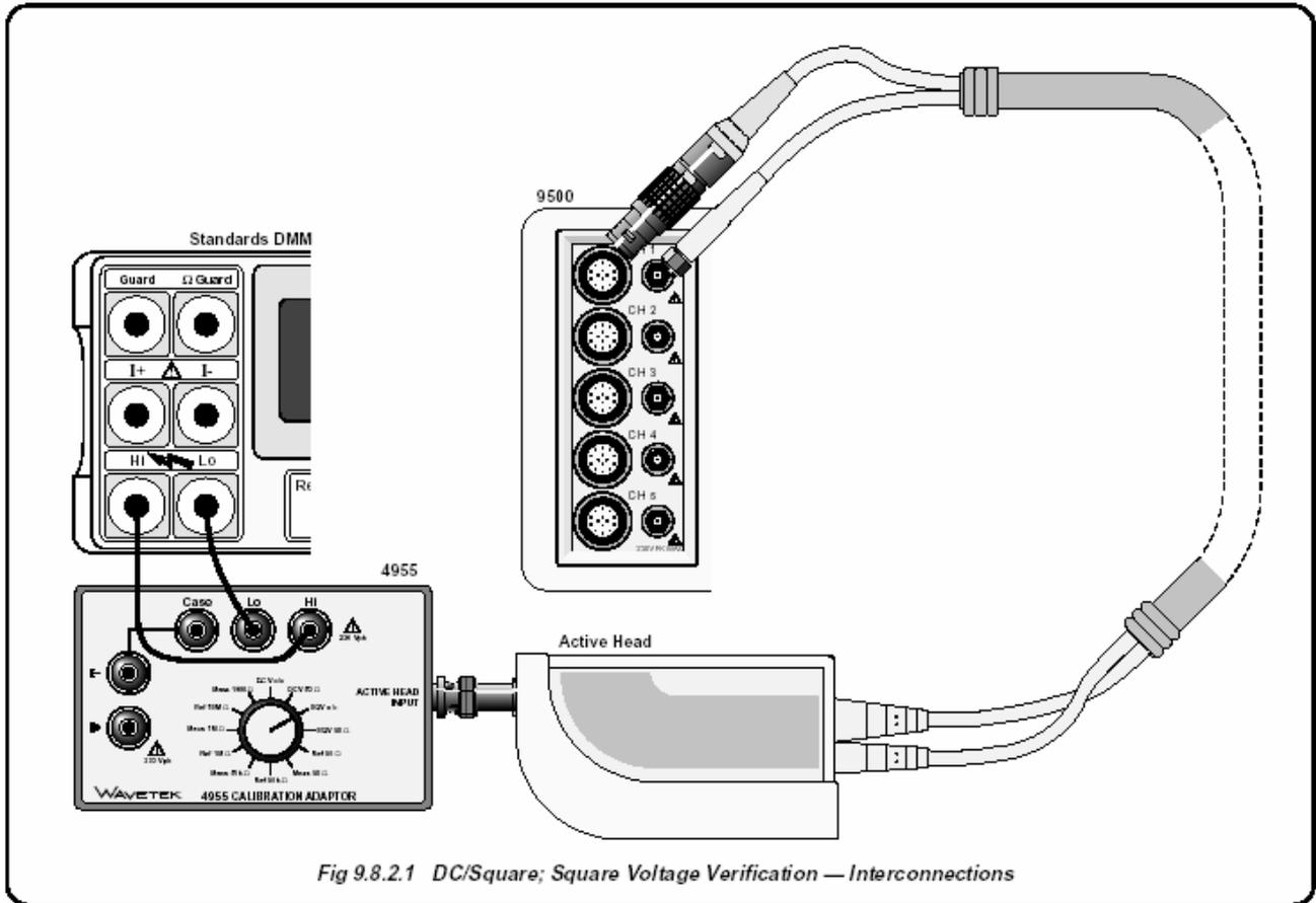
Fig 9.8.2.1 DC/Square; Square Voltage Verification — Interconnections
