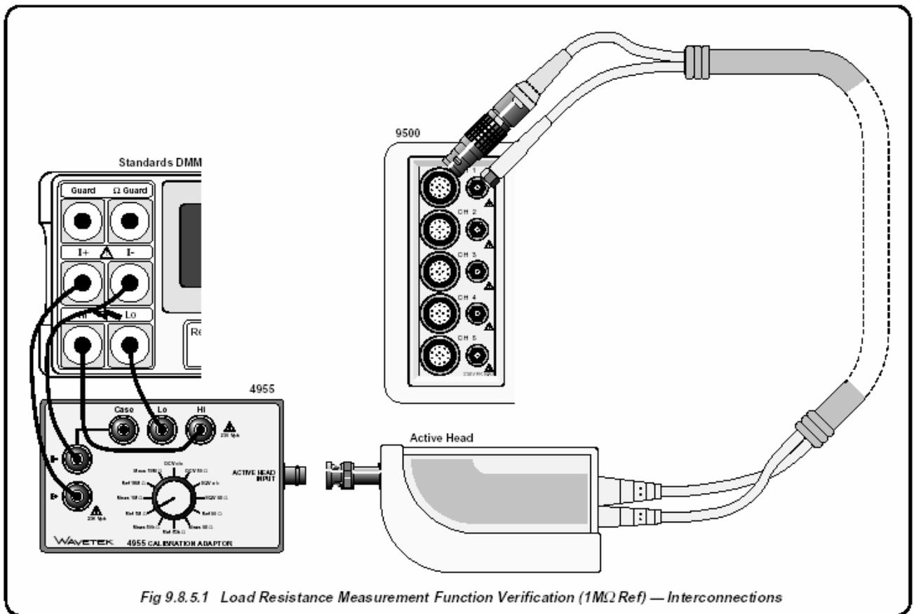
Fig 9.8.5.1 Load Resistance Measurement Function Verification (1MΩ Ref) — Interconnections
