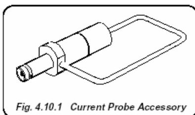
Fig. 4.10.1 Current Probe Accessory
