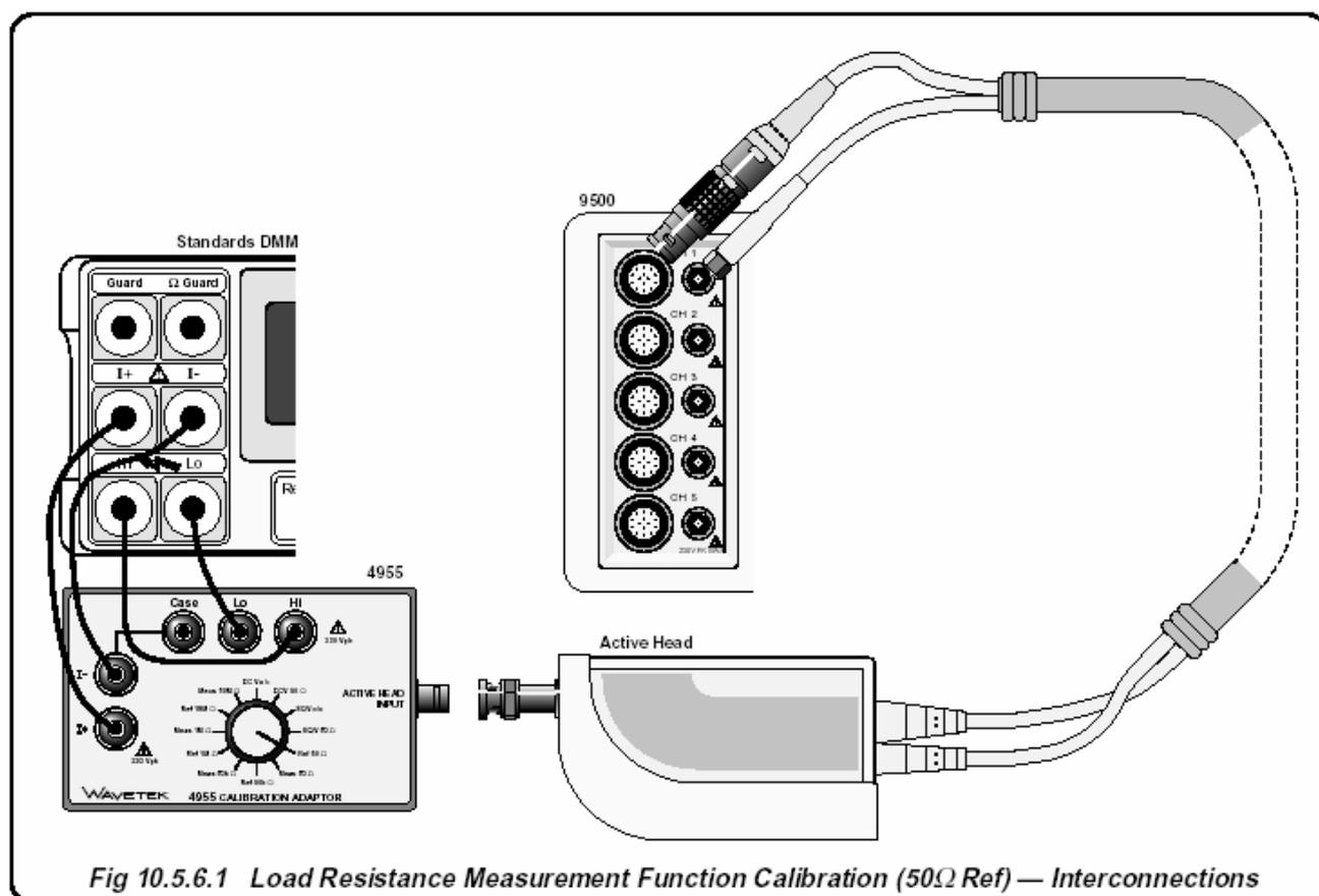
Fig 10.5.6.1 Load Resistance Measurement Function Calibration (50Ω Ref) — Interconnections
