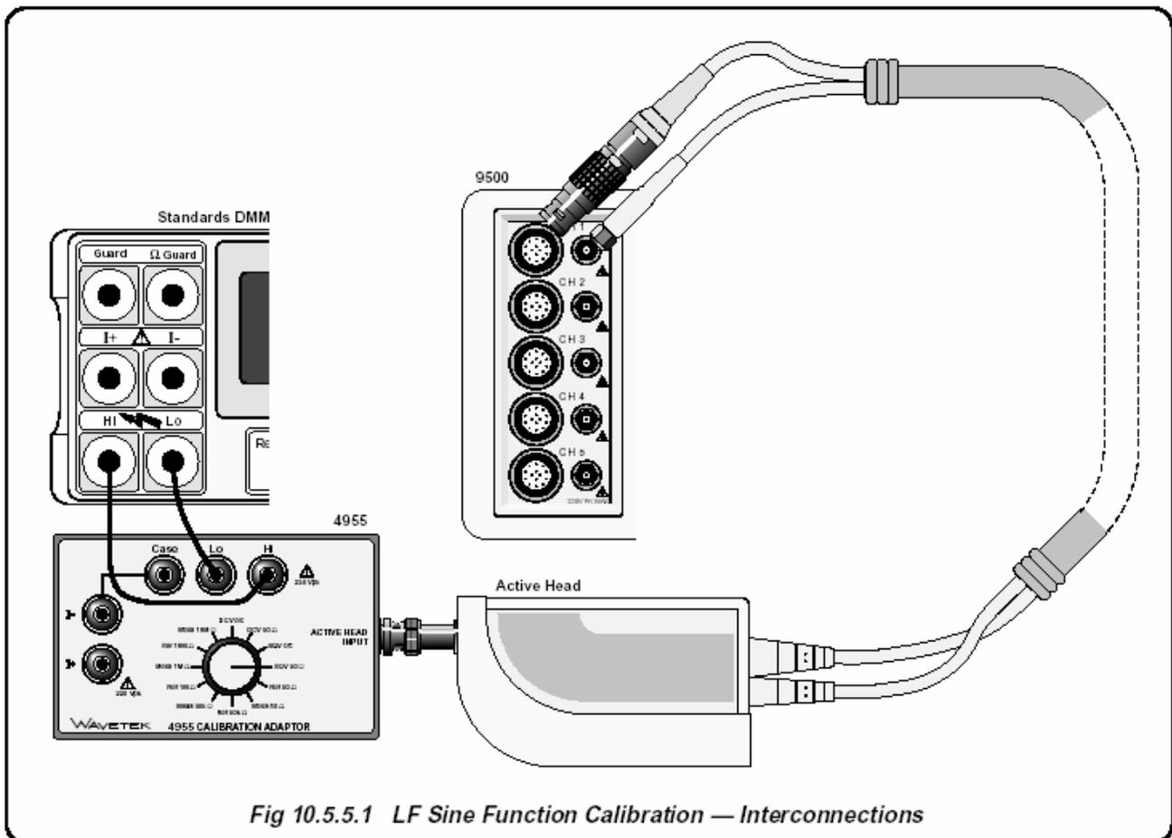
Fig 10.5.5.1 LF Sine Function Calibration — Interconnections
