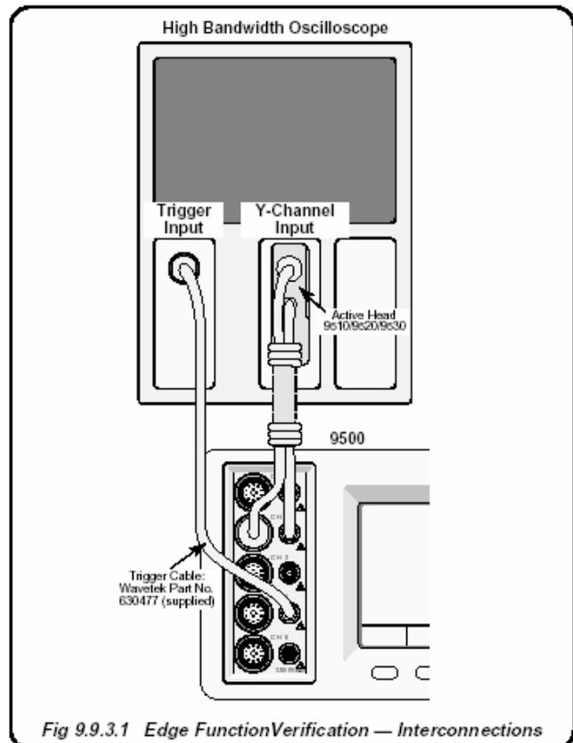
Fig 9.9.3.1 Edge Function Verification — Interconnections
