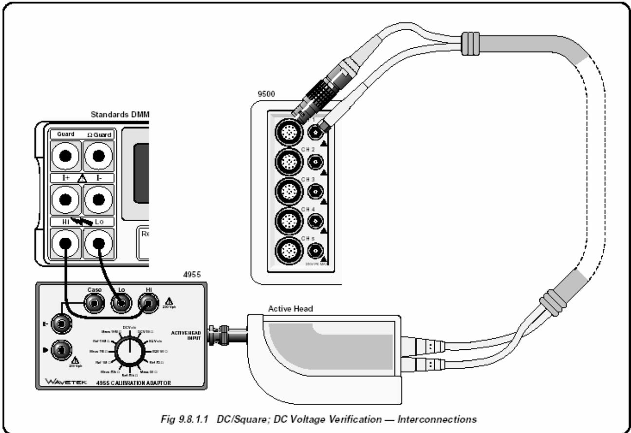
Fig 9.8.1.1 DC/Square; DC Voltage Verification — Interconnections
