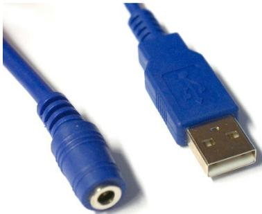
Connect the long, blue power cord of the docking station to the included 5.5V adapter of the SPECTRAN V5 and **connect the adapter to your power supply**. Now connect the long, blue MASTER-USB cable of the docking station to your PC (if available /desired) - ready.
