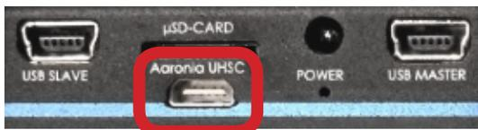
The Aaronia UHSC port allows direct access to the SERDES outputs / inputs of the ECP3 FPGA SPECTRAN V5. These provide extremely fast data transfer of up to 4x3GSPS.
