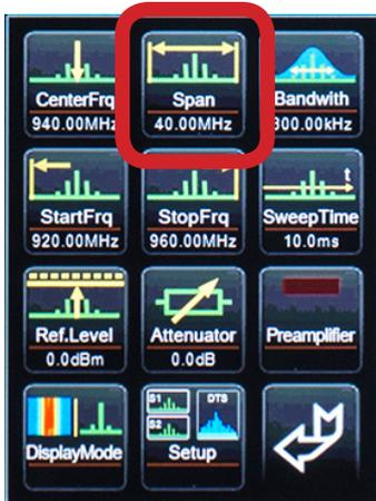
Span determines the frequency range for the measurement. The afore mentioned center frequency is not affected. Instead in case of changes to the span, the „Start/Stop-frequency“ will automatically be adjusted to retain the Span. The Span function is comparable with a „magnifier function“, which, however, only works on the X axis.
