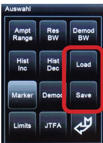
With Load and Save you can save up to 10 individual soft displays in the memory of the SPECTRAN. Here different parameters of the soft displays (also for a two- or four-fold constellation) are saved. This data will be saved for each soft display:
