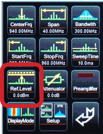
The reference level sets the position of the displayed signals relative to the top of the screen in dBm. The lower the setting (e.g. -20dBm), the closer to the noise and the more interfering signals will be visible.
