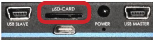
With our special  $\mu$ SD cards, you can record up to 64GBs or 128GBs of measurement data inside the analyzer. The  $\mu$ SD card works under FAT32 and can thus be directly read on a PC via the included adapter.
