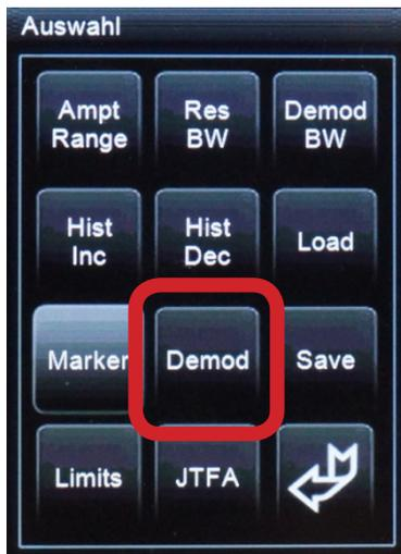
The demodulator makes pulsing & modulations up to 10 kHz audible and allows for „eavesdropping“ of individual signal sources (such as radio stations, two-way radios, etc.).
