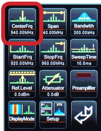
Displays the frequency in the middle of the screen. In case of changes to the middle frequency, the span parameter will be adopted. Advantage: Quick check of different frequency ranges with identical span and without changes to the start-/stop frequencies.
