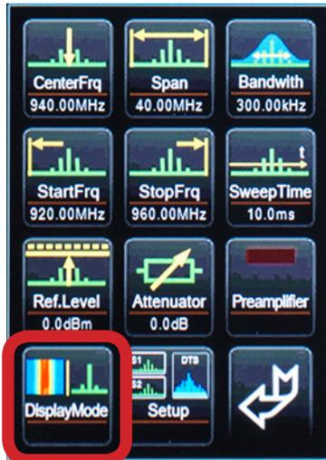
In display mode you can choose between the main modes „DTS“ (real time mode) and „Soft“ (sweep mode) respectively. For each of these two modes you can also select a separate display type and the number of windows (only in soft mode).
