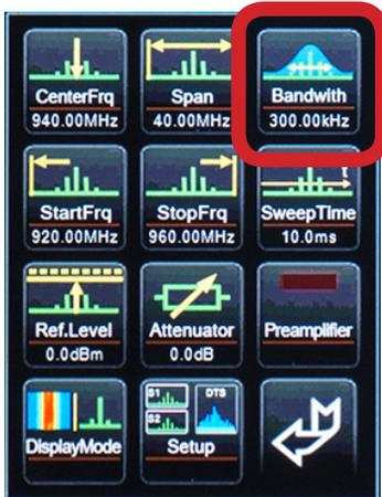
Bandwidth (Bandwidth) simultaneously sets the level of detail and sensitivity. **In real time mode this function cannot be set manually, instead the bandwidth is calculated automatically from the Span. The formula here is  $\text{Span}/220 = \text{Bandwidth}$ . So for a Span of 44MHz the bandwidth corresponds to 200kHz.**
