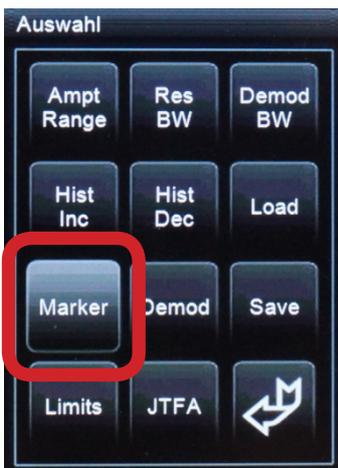
With the cursor you can exactly determine the frequency of single signals in the spectrum.
