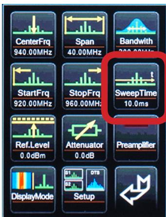
Determines the measurement period. The higher the sweep time the more accurate the measurement, but the longer the measurement period.
