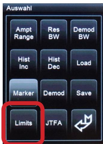
With „Limits“ you can define a maximum („Max“) or a minimum („Min“) level value (in dBm), which will be applied to the complete spectrum. With the „Limit On“ button you can turn the set limits on and off.
