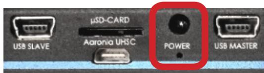
Standardized 3.5mm mono „jack“. The input voltage must be between 5V and 5.9V DC (direct current). The included power supply provides a voltage of 5.5V at up to 6A (33W).
