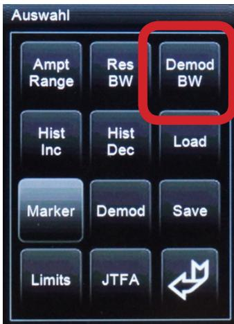
The demodulator bandwidth allows a clearer demodulation of individual signals. With it, the demodulation bandwidth can be adjusted according to the signal width. For FM for example you should select a rather high bandwidth of about 500kHz, for AM, the bandwidth can be considerably narrower (for example, 20 kHz). Ultimately you will have to experiment to find the perfect bandwidth for each demodulation.
