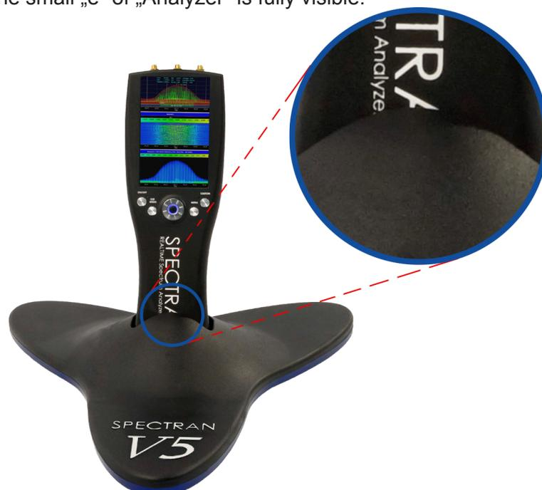
**NEVER** force the device into the docking station. A little bit of pressure and some slight back and forth movements might be needed until the device is fully locked into place, as shown above. Please make sure that the device is placed correctly into the docking station!
