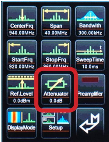
The attenuator (built in) attenuates any fed signals by the corresponding dB value to avoid an overload of the RF input.
