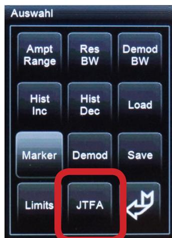
With „JTFA“ you can adjust the real time measurement according to your requirements. Here you have direct access to the symbol processing and can for example suppress unwanted signals already in the run up. The following are available:
