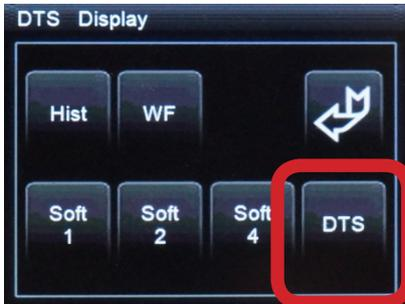
In the real time mode „DTS“ around 50,000 symbols per second are calculated and graphed. Here, there are two display modes available:
