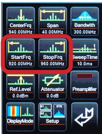
StartFrq (Start frequency) determines at which frequency the measuring range should start, while StopFrq (Stop frequency), determines at which frequency the measuring range should stop. This results in the entire frequency range (Span), which is measured.
