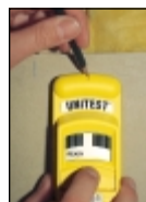
Accurate location of materials (e.g. joist, stud, etc.)
