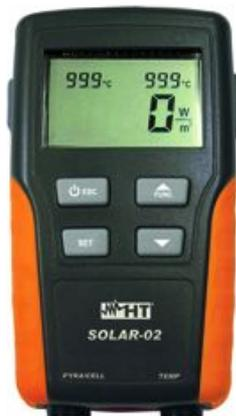
SOLAR-02 remote unit permits also to display the irradiance and temperature values independently (ideal solution during a pre-test on installations) besides test/recording through SOLAR I-Vw
