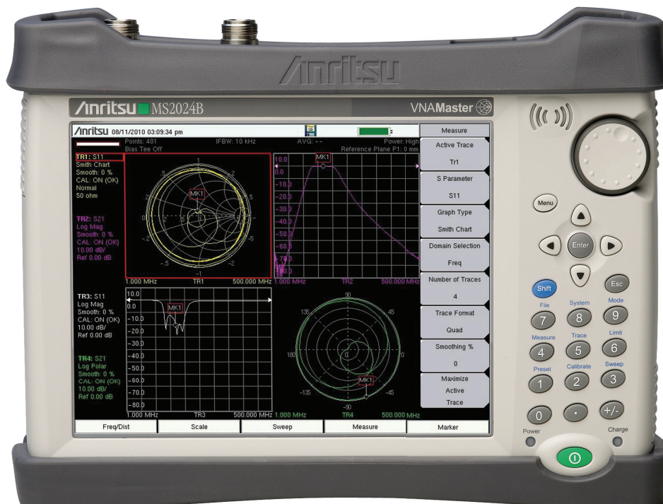
VNA Master™ MS202xB/MS203xB Vector Network Analyzer + Spectrum Analyzer Compact Size: 199 mm x 273 mm x 91 mm (7.8 in x 10.7 in x 3.6 in), Lightweight: 3.5 kg (7.6 lb)
